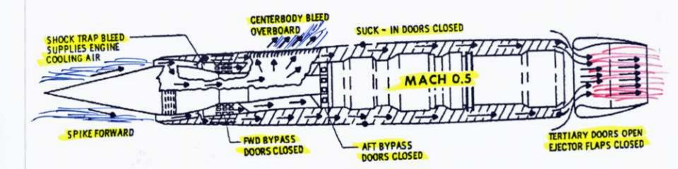
Low supersonic airflow – Spike locked forward, suck –in doors and tertiary Doors closed. Ejector flaps opening depending on engine thrust pressure & forward bypass doors modulating as required
