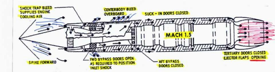
RAM THRUST EFFECT starting to become noticeable- Spike translating aft as speed increases, Aft Bypass probably 15% open & Forward Bypass modulating. Ejector Flaps now further open
