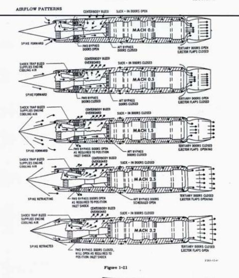
No Air Movement – Spike locked forward, most doors open to get extra air to engine. AFT Bypass doors & Ejector Flaps closed
