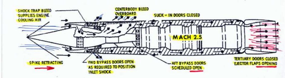
Design Top Speed -Inlets tight – Spike full aft, Aft Bypass doors closed, Forward Bypass just barely modulating, ejector flaps normally full open
