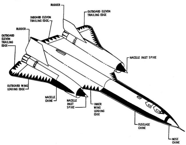
Figure 4-5. Composite-Honeycomb Areas of the SR-71
